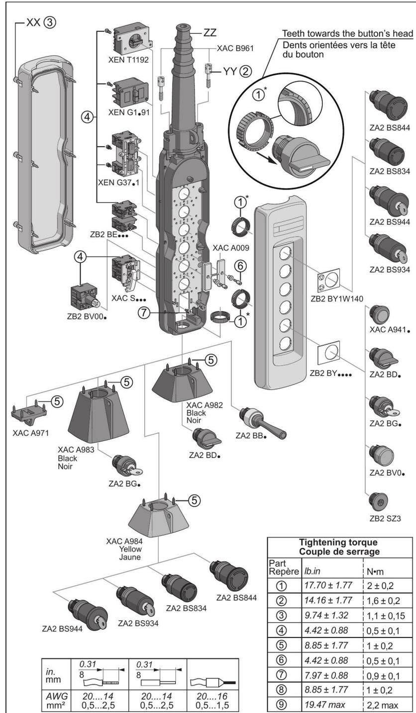
**With emergency stop trigger action and mechanical latching pushbuttons**
